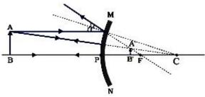
Use of convex mirror—as rear view mirror in vehicles Why—always gives erect image with large field of view 1 1/2 1 3
